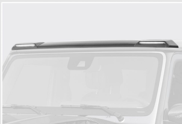
17. Roof LED panel
