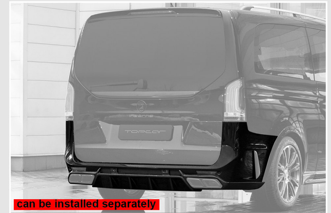
11. Rear bumper for painting with diffuser
