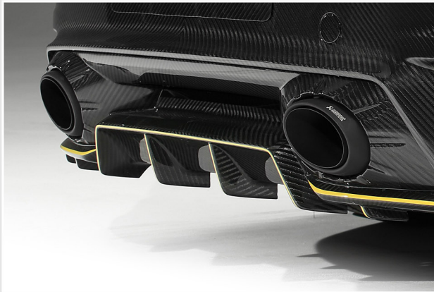
Titanium exhaust ( Akrapovic ) with black tips
