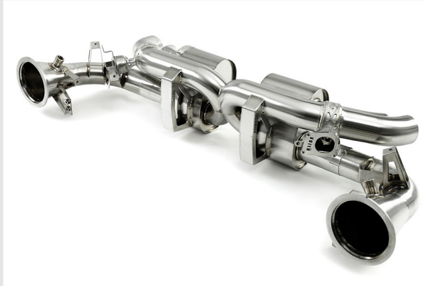
Inconel exhaust (Kline) - Valvetronic silencer section
